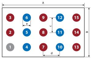
Pad 1 is Gate: Pads 2, 3, 7, 8, 9, 13, 14, 15 are Source; Pads 4, 5, 6, 10, 11, 12 are Drain;
