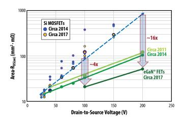
Figure 1: EPC's fifth-generation technology cuts the die size in half for the same on-resistance and voltage rating
