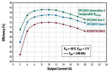
Figure 3: Gen 5 Devices have higher performance and are about half the size of Gen 4. Both Gen 5 and Gen 4 are far superior to the best available MOSFET.
