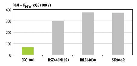
Figure 2: Page 5 from a presentation given at the International Conference on Integrated Power Electronic Systems (CIPS) in Nuremberg, Germany in March 2010 showing the comparison between EPC's first generation EPC1001 and the best available MOSFETs.
