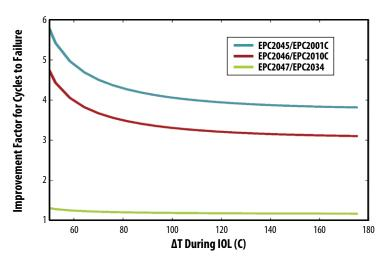
Figure 5. Shown is the relative power cycling performance of Gen 5 devices compared with Gen 4. Smaller die sizes have less differential thermal expansion with the underlying PCB, thus reducing strain during thermo-mechanical cycling.
