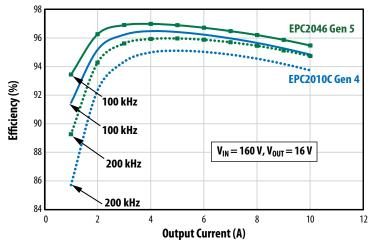
Figure 4: Comparison of efficiency of 200 V eGaN FETs from Gen 4 and Gen 5 at 100 kHz and 200 kHz. Despite being half the size and having the same on-resistance and voltage rating, the Gen 5 devices outperform Gen 4 by a wide margin.
