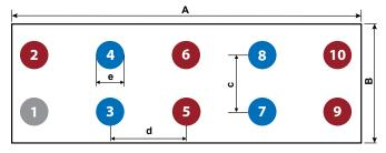
Pad 1 is Gate; Pads 2, 5, 6, 9, 10 are Source; Pads 3, 4, 7, 8 are Drain;
